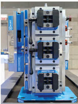
A Kurt Caged Tombstone loaded with 3 PFW vises and 96 mm bases and a DX6 mounted with pull studs to a quick-change base.
