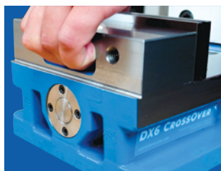
Through body chip evacuation &amp; integrated handle
