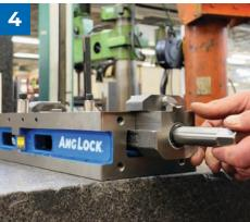
**Install new nut and screw:** clean the vise body, lubricate contact surfaces, and insert the new TL6-3-SA nut and screw assembly.
