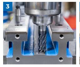
**Rotate the vise:** Clean up the vise after removing the nut stop and rotate the vise 180° so the four tapped holes are facing the operator.
