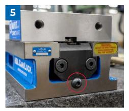
**Install nut and screw assembly stop:** rotate the vise 180° and install short shoulder screw in the tapped center hole as shown above.
