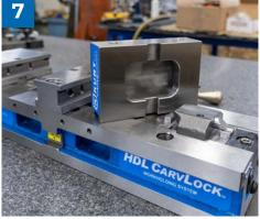
**Install CarveSmart Jaws:** use original shoulder bolts to install stationary jaw, snap movable jaws on to each nut.
