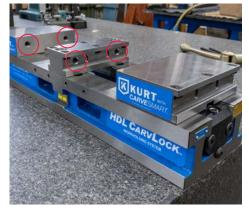
**PRO TIP:** If you still need to use non-CarveSmart Kurt jaws, just rotate the movable jaw 180° and use standard cap screws. Cap screws can also be used on the center stationary if necessary.
