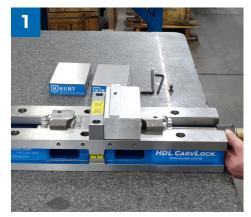
**Remove Jaws and Nut and Screw:** Strip down the HDL6 by removing jaws and nut and screw assembly from the vise. Clean the vise body.
