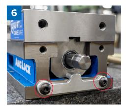
**Install nut and screw retainer stop:** rotate the vise 180° and install the retainer bracket using the long screws in the bottom holes as shown.
