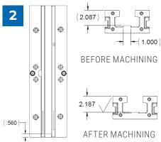
**Machine off nut stop:** Refer to dimensions. The New machined surface **must match** the original with a minimal step between them.
