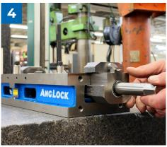
**Install new nut and screw:** clean the vise body, lubricate contact surfaces, and insert the new TL6-3-SA nut and screw assembly.
