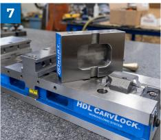
**Reinstall Jaws:** use original shoulder bolts to install stationary jaw, snap movable jaws on to each nut.
