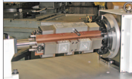
Solution: Eight station indexing trunnion fixture for high speed machining.
