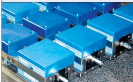
Solution: Bushed and tapped sub-plate allows fast vise repositioning.
