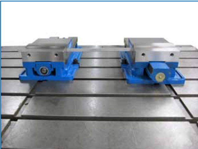
D675 Nut Protrudes when all the way closed.
